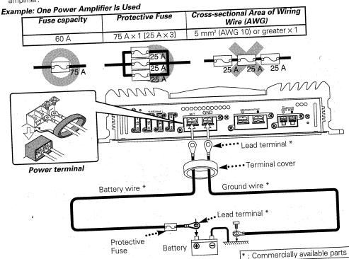
Pass battery and ground wires through supplied terminal cover and connect to respective Power terminal terminals. After completing connections, fasten terminal cover over terminal bracket.
